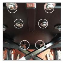
2 Further adjustment might be available by altering the position of the drop hooks on the wheelbase and/or the polypropylene base board. If fitted to a powerchair, it may be possible to adjust the wheelchair push handles towards the rear to allow create additional seat depth.
