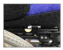
3 Fit the lock at the rear. Do not tighten as you will be adjusting these later. Use the drop hook brackets to ascertain a good position and check for obstacles on the frame
