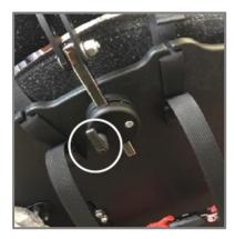
To adjust the depth position and angle of the headrest loosen the headrest bolts. Adjust to the required position. Tighten up bolts when the desired position is achieved.
